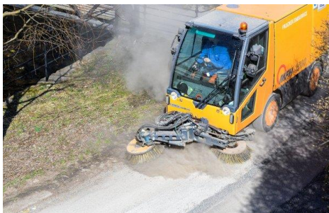
Figure 3.6 Sweeping of roads in Oslo (Photo: Knut Opeide, Statens vegvesen). Snow deposition
