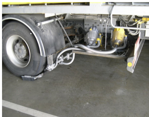
Figure F1. Photograph of an on-road tyre wear collection system using an aspiration system with a slot-type capture hood attached to the rear left axle of a truck. Reprinted from Kreider et al. (2010) with permission from Elsevier.
