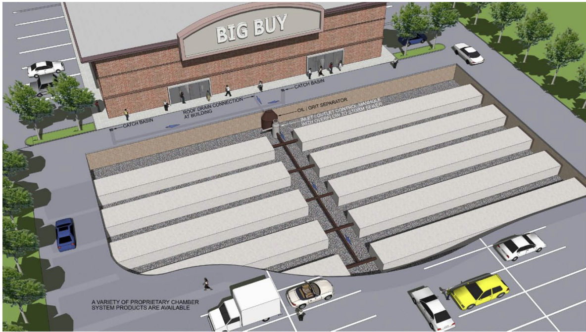
Figure 6.12 Schematic design of an infiltration chamber system below a parking lot (CVC and TRCA 2010)
