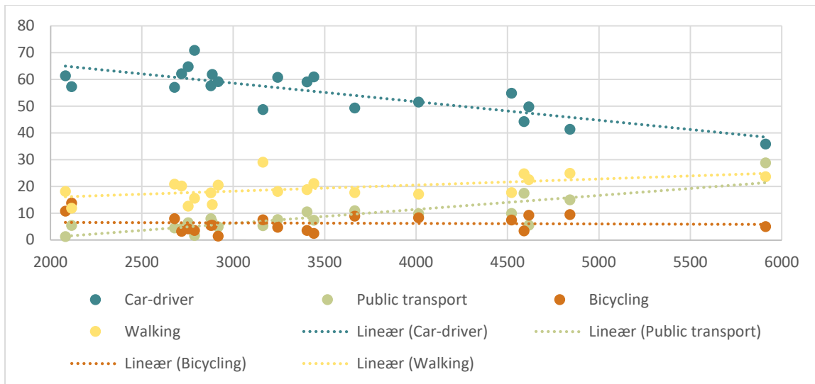
Figure 6: Modal splits versus city densities in the 20 case cities of various sizes. Percentages, of all daily journeys starting and/or ending within the cities made by different modes on the y-axis, and densities (population plus workplaces per km 2 ) on the x-axis.
