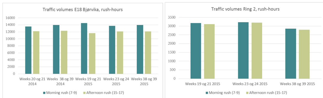
Figure 6: Average traffic volumes per workday in rush-hours in the morning (7.00 – 9.00) and the afternoon (15.00 – 17.00), total for both directions, number of vehicles. The capacity reduction in the Smestad tunnel was implemented week 23, 2015.
