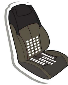
Figure 3. Illustration of the vibrotactile seat and the location of the 48 vibration motors (i.e., white circles). The motors are arranged in two matrices of 6x4 motors (one matrix in the seat back, the other matrix in the seat bottom).
