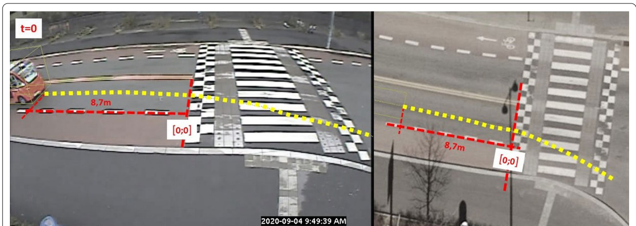
Fig. 5 The first traceable position of the shuttle in camera angle #2 ( t = 0 , distance = 8.7 m), the axes for distance measurements (red lines) and the trajectory of the shuttle (yellow line)
